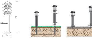
Fixing Minilite into the ground
