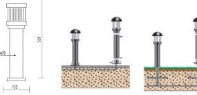
Fixing Minilite into the ground
