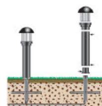
Fixing Minilite into concrete (or masonry elements)
