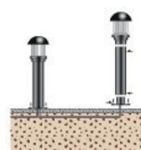
Fixing Minilite into concrete (or masonry elements)
