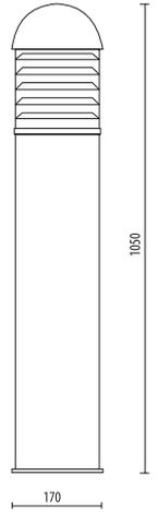
BOLLARD with post and round lid in resin material
