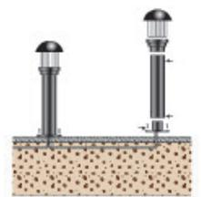
Fixing Minilite into concrete (or masonry elements)
