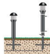
Fixing Minilite into concrete (or masonry elements)
