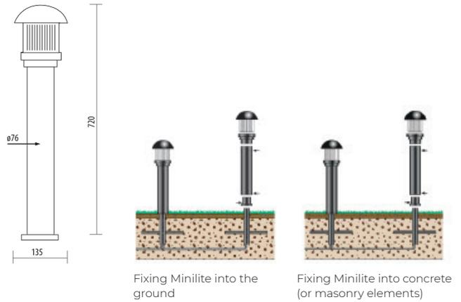
Fixing Minilite into the ground
