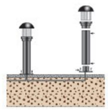
Fixing Minilite into concrete (or masonry elements)
