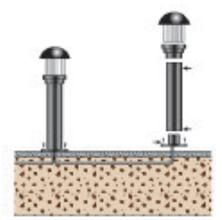
Fixing Minilite into concrete (or masonry elements)
